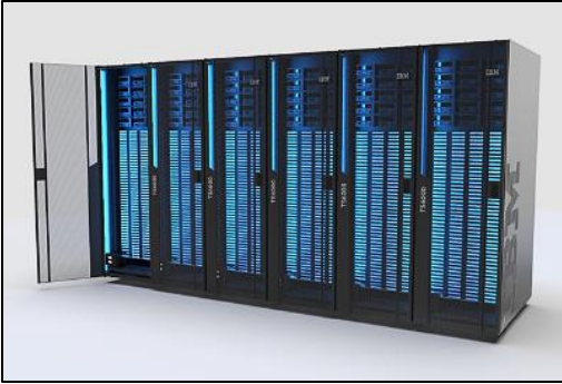
Figure 5 – The IBM Diamondback Tape Library delivers ultra-high data density, with up to 27.9 PB of native data in a single eight-square-foot library using LTO Ultrium 9 cartridges.
